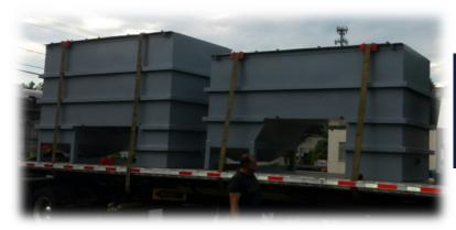
Clarifier Separators designed to remove settable solids, suspended solids, and free and dispersed oil in one unit
