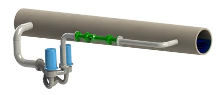
For high flow rates where storage is not an option, Theia offers an inline treatment system that aerates, oxidizes and can neutralize the water. Additionally metals and nutrients can be precipitated at very low costs with a natural additive. Polymers can be mixed into the water to allow for settling or filtration
