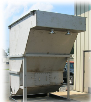
Precipitation & Settling of Solids through Clarification
