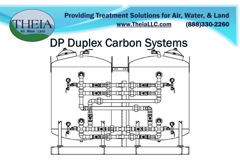
The DP series consists of a pair of our LP or AC series vessels, skid mounted with a full manifold. Manifold allows for a single inlet and outlet for two (or more) vessels. The System can operate with either vessel in lead or lag, and can isolate either vessel for change out or backwash.
